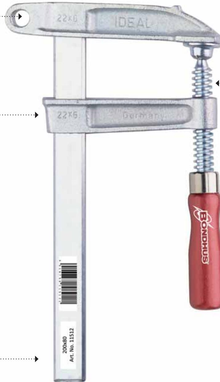
Swiveling steel pressure plate and high quality, smooth turning Acme thread spindle create more clamping power with less effort
