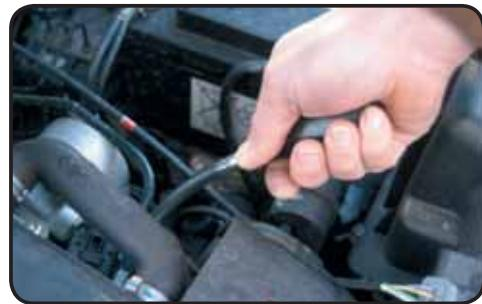
Hexagon Nutdriver with flexible shaft, with plastic jacket
